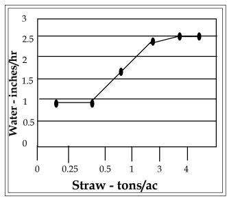
*Figure 3.* Effect of straw rate on water infiltration on a silt loam soil (7).
